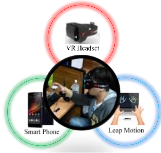
Figure 4. The low-cost head-mounted 3D interactive system construct proposed in this paper.
