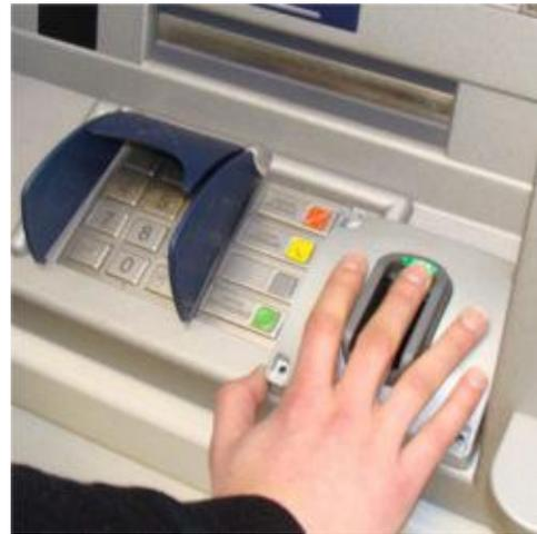
Fig. 1. Biometric (Fingerprint scanner) ATM. (Image Source: <http://cacm.acm.org/news/95831-biometric-atm-gives-cash-via-finger-vein-scan/fulltext>)
