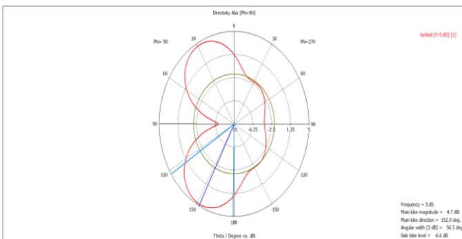
Fig. 4. Simulated directivity at 5.8 GHz resonant frequency
