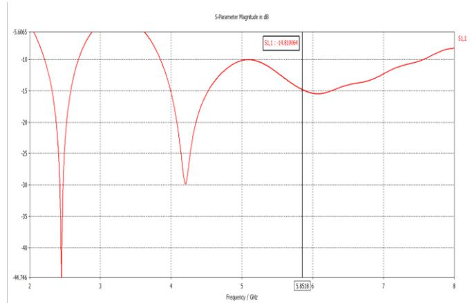
Fig. 5. Simulated Return Loss at 5.85 GHz resonant frequency
