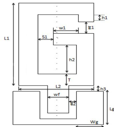
Fig. 1. Geometry of the Proposed G-shaped Antenna
