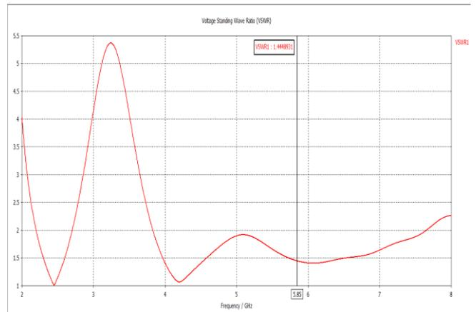
Fig. 6. Simulated VSWR at 5.85 GHz resonant frequency
