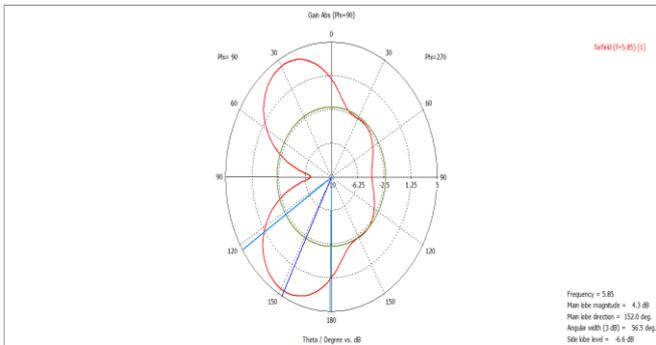
Fig. 3. Simulated gain at 5.8 GHz resonant frequency
