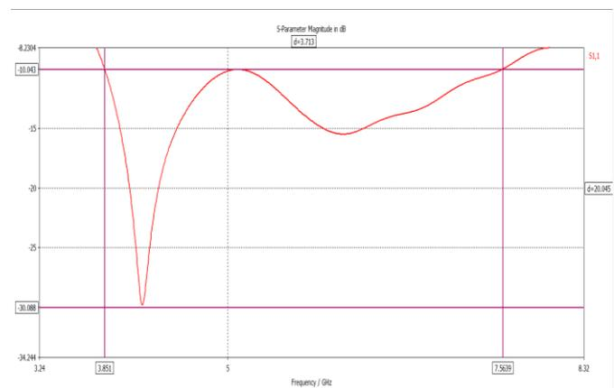
Fig.1. Simulated bandwidth at 5.8 GHz resonant frequency
