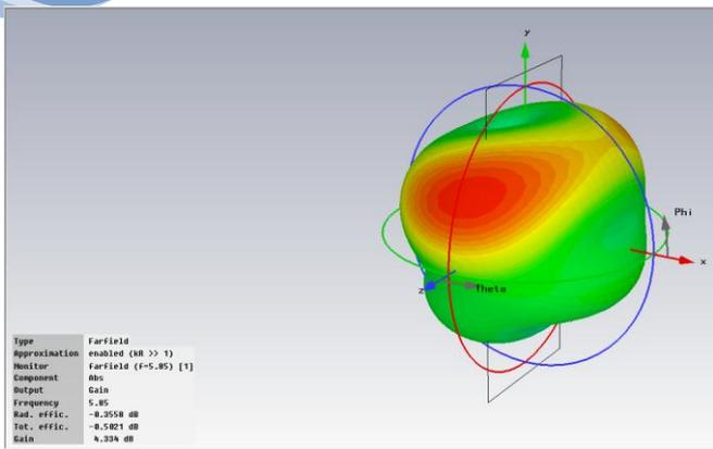
Fig. 2. Simulated radiation pattern and gain at 5.85 GHz resonant frequency
