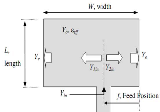
Fig. 2. Geometry of length and width
